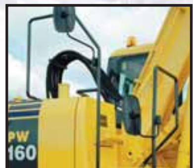
Large handrail for safe access
